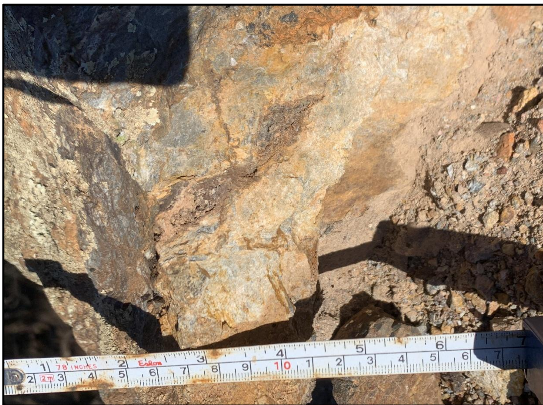
Photo 2: Advene Prospect, silicified & brecciated metasediments with Fe-oxide lenses
