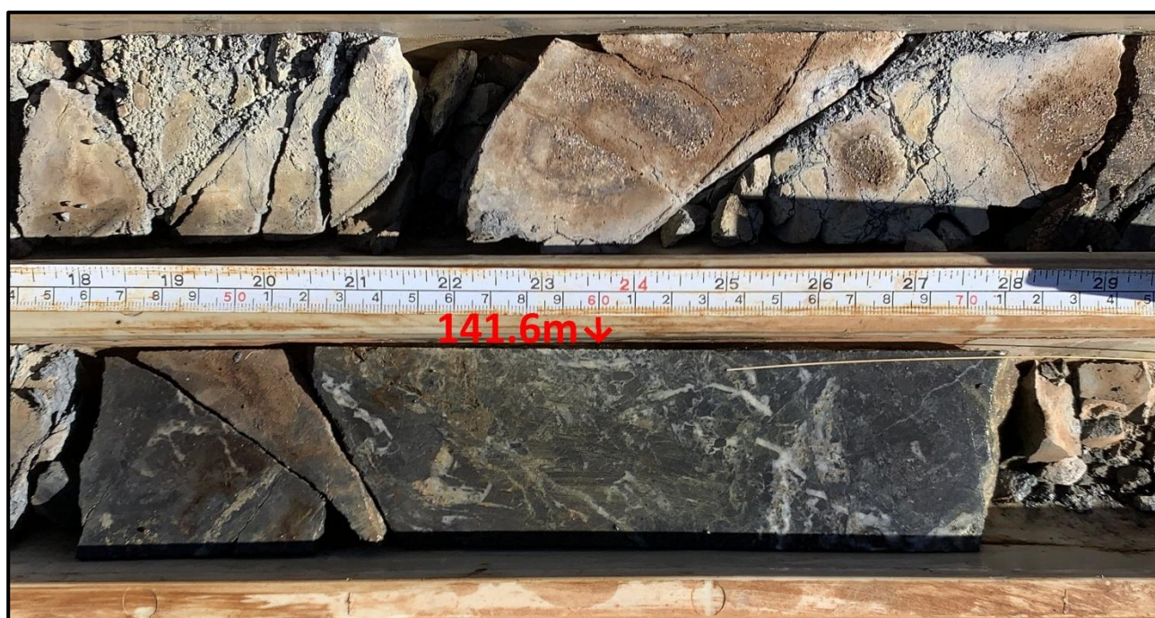
Photo 13: DD14AV005, 141.6m, silicified & brecciated sediments with quartz veinlets and pyrite
